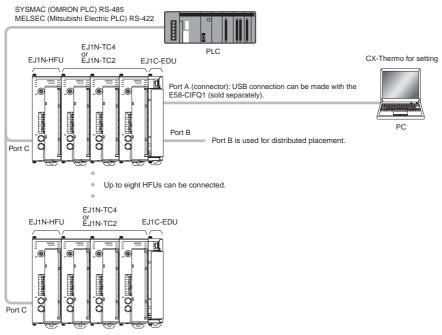
Note: Set the EJ1N-TC to a communications unit number that is not being used by the EJ1N-HFU.
