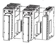
Note: 1. Do not connect the End Unit directly to an HFU.
