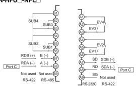
RS-485 for port C and RS-232C can be switched. A separate EJ1 model must be used for RS-422 communications.
