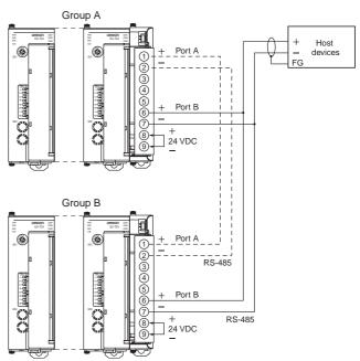
Note: Wire the dotted line when settings for all distributed Units are being made from one port A connector.
