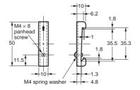
**Note:** Two screws are included with the EJ1C-EDU for the End Plate. Always attach End Plates to both sides.
