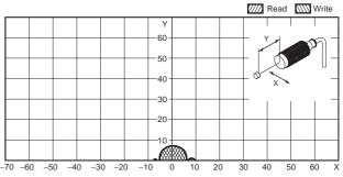
V680-HS51 (embedded in metallic material) & V680-D2KF52M (embedded in metallic surface: steel)
