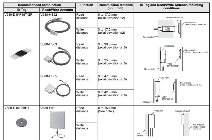
Note 1. When mounting the V680-HS65, be sure to attach the Mounting Brackets at the base of the Antenna.
