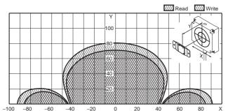
V680-HS63 (mounted on non-metallic material) & V680-D1KP66MT (flush-mounted on metallic surface: steel) V680-D1K66MT (flush-mounted on metallic surface: steel)
