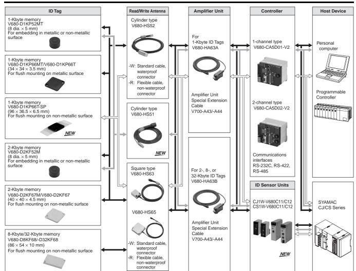
Note 1. Use a V680-HS51/-HS52 Antenna if the V680-D1KP52MT or V680-D2KF52M is to be embedded in metal. Communications cannot be performed if a V680-HS63 Antenna is used in combination with the V680-D1KP52MT or V680-D2KF52M.
