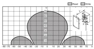
V680-HS63 (mounted on metallic material) & V680-D8KF68/-D32KF68
