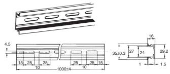
$^{\star}~$  A total of twelve 25  $\times$  4.5 elliptic holes is provided with six holes cut from each track end at a pitch of 10 mm.
