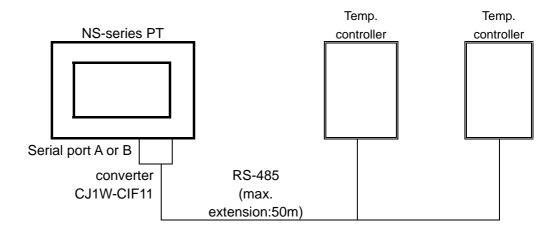
By using another communications port, you can simultaneously connect temperature controllers and a host. With one more serial port, NS can connect PLC, barcode reader, Memory Link and can communicate with NS-Designer.
