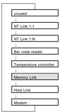
After you have thus set communications to Memory Link, use the **Details** key to set the communications conditions for the Memory Link connection (for details, refer to section 2.2). However, with system menu you cannot set the **Notice start \$B** and **Notice start \$W**.
