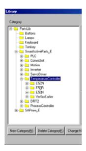
Temperature controller is grouped by model, channel and broadcast. For each operation instruction, a Smart Active Parts part is available.
