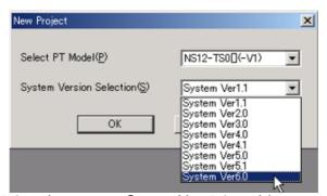
In NS-Designer Ver. 5.0 or later open SystemVer.5.0 and later project, click **Settings** – **System Setting**. Select tab '**Comm.**– **All**' and set Serial Port A (or Serial Port B) to **Memory Link** (select from the pull down menu).
