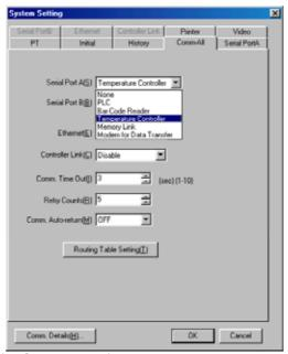
Select tab Serial Port A (or Serial Port B) and set baud rate.
