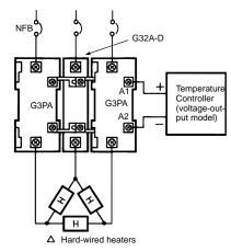
Note: When performing 2-wire switching of 3-phase power, the leakage current that is generated when the SSR with the shorted phase is turned OFF will increase by a factor of 1.7.
