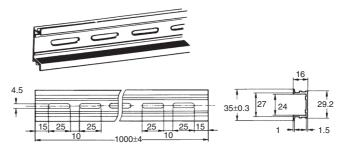
A total of twelve 25 × 4.5 elliptic holes is provided with six holes cut from each track end at a pitch of 10 mm.
