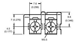
Allow suitable slack on leads when wiring, and do not subject the terminals to excessive force. Maximum tightening torque is 10 kgf-cm (72.50 ft-lbs).
