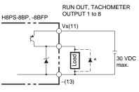
\* When using an inductive load, connect a reverse surge-absorbing diode.
