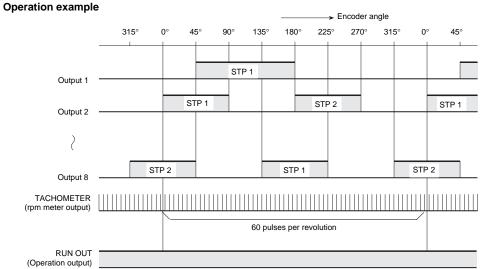
ON during run mode and test mode
