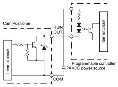
+COM RUN OUT 24 VDC -COM Programmable controller
