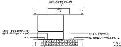
FORCED RUN (input terminal for signal forcibly operating the Rotary Positioner)
