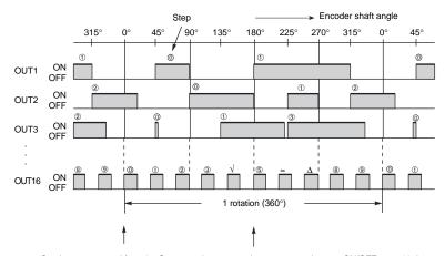
Can be programmed from 0°. One control output can be programmed to turn ON/OFF up to 10 times.
